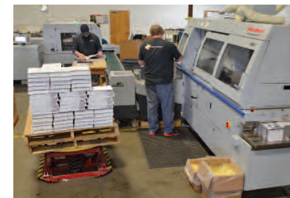
The new perfect binding and trimming solution can bind and trim books up to 2.5" thick which is critical for the jobs at BR Printers.
