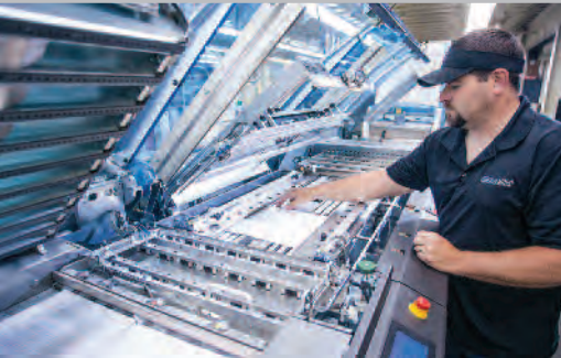
An EBSCO Media technician makes final adjustments to the Standard Hunkeler Cut/Stack system before running the next job...
