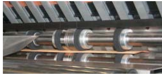
Scoring with 1-1/8" slittershafts
