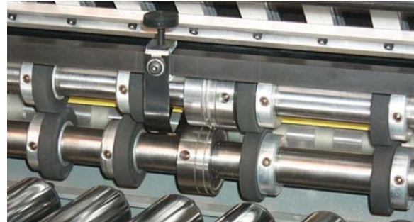
Fig. 7 Perforating on 1-1/8" slittershaft
