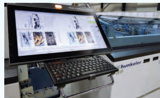
Premiering in the Hunkeler booth was a multi-purpose Hunkeler/ Horizon combination finishing line producing either stacked or folded output from a paper roll. Web Inspection (above) ensures accuracy.
